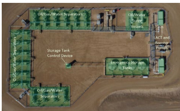
Figure 3: A production facility using a tankless design
